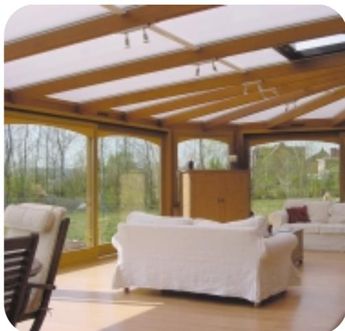
**Polygal Thermogal** unique inner X-brace structure provides extra-strength, rigidity and outstanding insulation. Available in different thicknesses, widths and colors. Ideal for low-pitched roofs and for glazing in closed structures with large-span openings.
