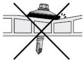
Incorrect - Non-perpendicular drilling and insertion
