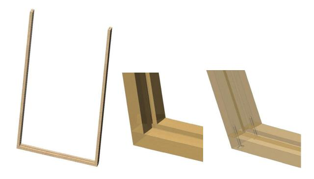
Step 3. Place UP 16 Edge Profile on both open edges of 16mm 48"x96" sheet
